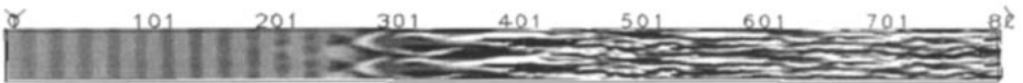
Figure 8 Same simulation as in Figure 6. Shown is the longitudinal velocity in a horizontal plane 10.3 wall units from the plate.
