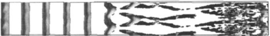
Figure 6 FSF simulation of a weakly compressible boundary layer on a flat plate. The longitudinal vorticity (dark shading) and the pressure (gray) are shown. (Courtesy F Ducros 1995.)
